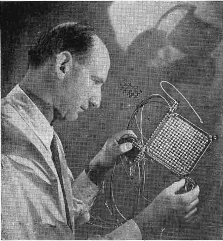
Dr. Jan A. Rajchman holds one of his Myriabit Magnetic Core Matrix Memory units which is capable of retaining 10,000 bits of information until needed.
